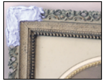
A close-up photo with mold displayed above one of the areas created with use of a pourable thermal strong dental casting material with simultaneous adhesive capabilities.
